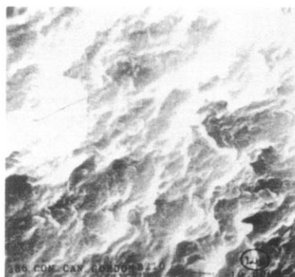
Figure 7 Scanning electron micrograph (10 000 X) of fracture surface (cross-section) of desiccated bottle of Figure 3
